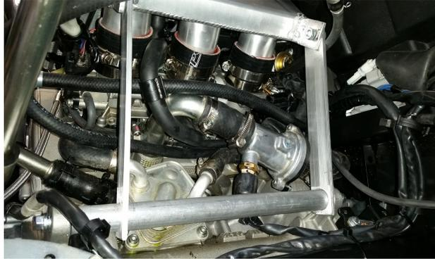
Install 3 supplied intercooler couplers on throttle bodies and clamp tight. Remove rubber cap from rear vacuum nipple on rear throttle body and push on the short vacuum hose from manifold kit as picture shows.
