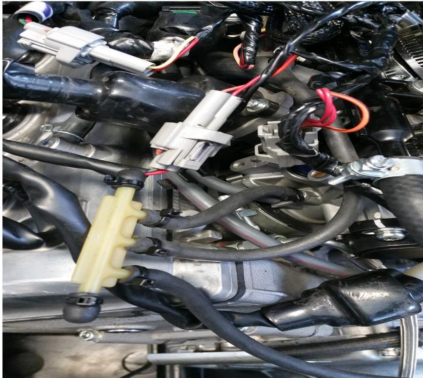
Connect one vacuum hose to PowerCommander map sensor and let the other hose hang behind engine.
